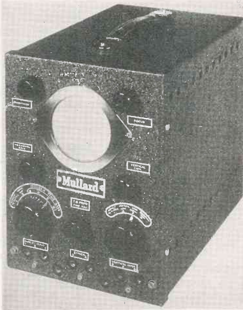
The Mullard type G.M. 3155 portable cathode-ray oscillograph employing a three-inch high-vacuum tube.
