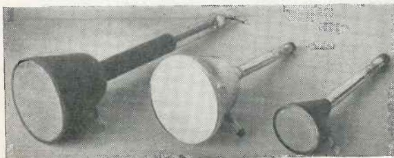
Fig. 10. (left) Three experimental projection tubes (20,000 v. 40,000 v. and 60,000 v.)
