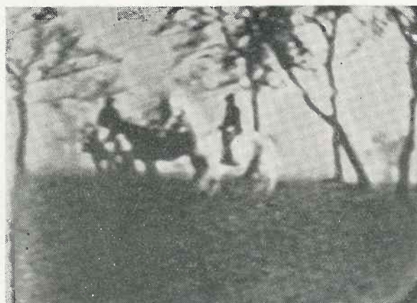
Fig. 2. The curious effect resulting when the oscillator is incorrectly tuned, coupled with an inadequate frequency response in the I.F. circuits.
